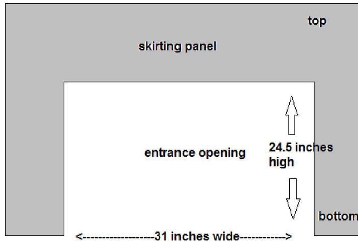
3. **Note:** When installing the door in a Thermal EverRock or Gorilla panel, you must remove both the front vinyl face of the panel and the foam backing when making your entrance opening. Additionally, 2 inches of foam must also be removed from the back of the panel along all edges of the entrance opening. This foam must be removed so that the door frame may be installed flush against the back of vinyl portion of the panel.
