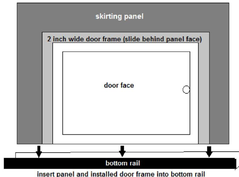
5. Install the entire panel (including the door) as you would install your other skirting panels. Insert the exposed bottom of the door frame into the bottom rail of your skirting system and fasten with screws. Re-insert door into door hinge.
